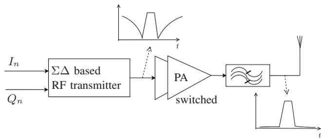
Fig. 2. Transmitters using  $\Sigma\Delta$  modulators
