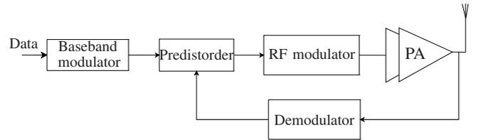
Fig. 5. Predistortion principle
