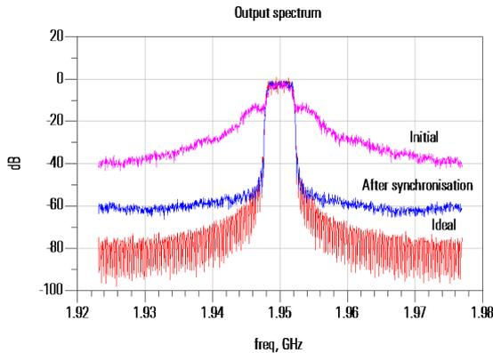
Fig. 6. Result of delay mismatch correction on the output spectrum
