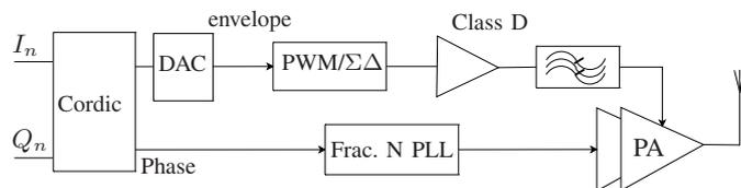
Fig. 3. Polar transmitter
