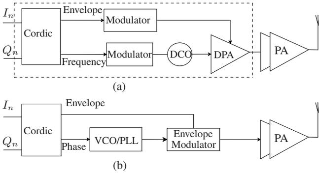
Fig. 4. Digital polar transmitters
