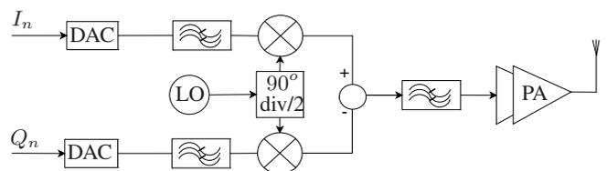
Fig. 1. I/Q ZIF transmitter
