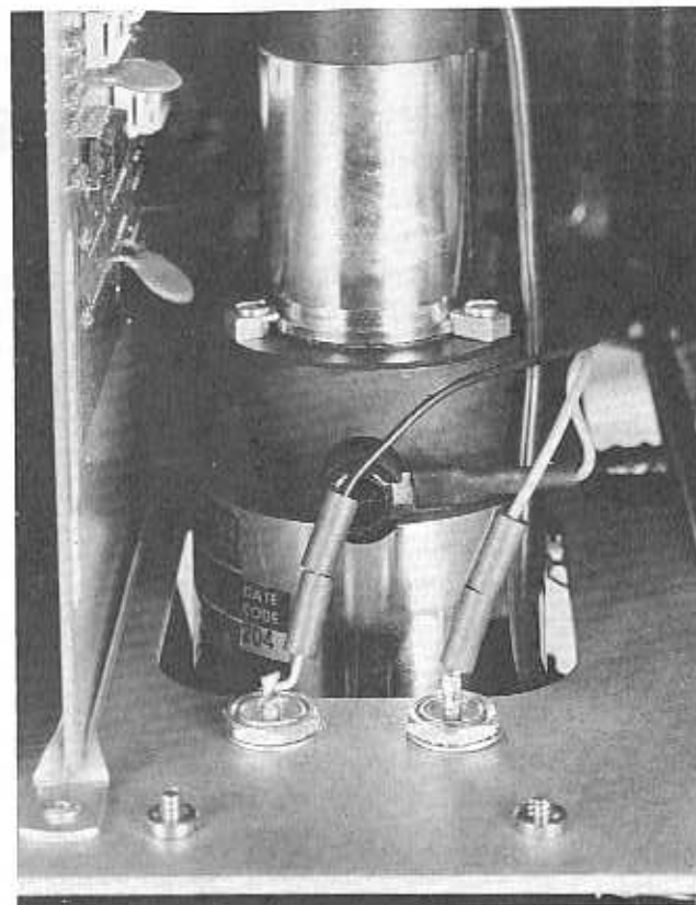
Figure 5-22. Ferrite beads and feed-through capacitors used to reduce motor commutation noise coupling to power leads.
