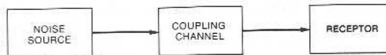
Figure 1-11. Before noise can be a problem, there must be a noise source, a receptor that is susceptible to the noise, and a coupling channel that transmits the noise to the receptor.
