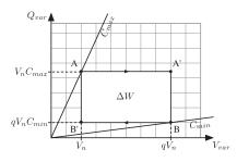
Fig. 2. QV-cycle for an e-KEH with a charge pump conditioning circuit that implements a fixed ratio q between the voltages biasing the transducer at its extremal capacitance values.
