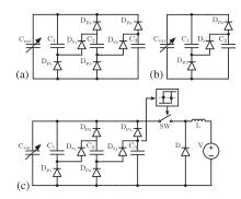
Fig. 7. (a) Simulated circuit, corresponding to the generic topology in Fig. 3, with N = 3. (b) Simulated circuit, corresponding to the generic topology in Fig. 3, with N = 2 (Bennet's doubler). (c) The circuit simulated with an implementation of the energy extracting interface.
