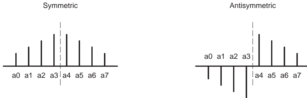
Figure 7–1. Symmetric and Antisymmetric FIR Filters
