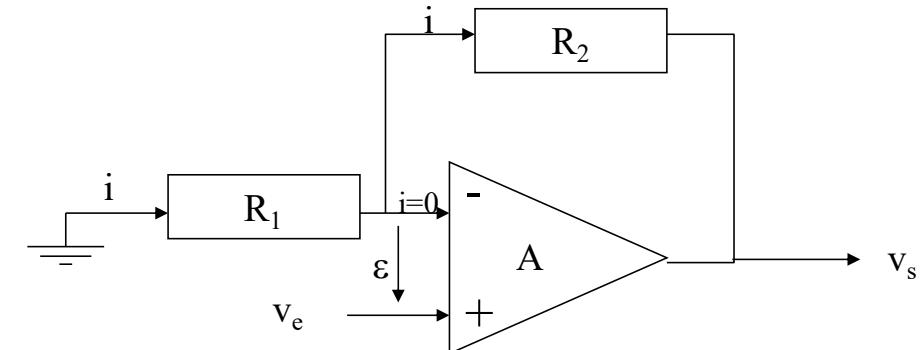
$$\Rightarrow \frac{V_s}{A} \cdot \left( \frac{1}{R_1} + \frac{1}{R_2} \right) + \frac{V_s}{R_2} = V_e \left( \frac{1}{R_1} + \frac{1}{R_2} \right)$$
