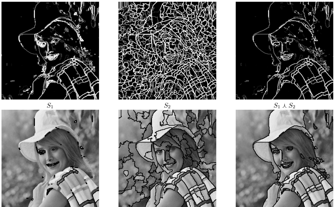
Fig. 5. Saliency maps obtained from Fig. 4 (first row) and associated segmentations into 100 regions (second row) [see text].
