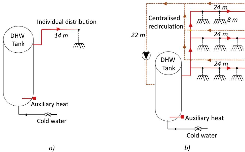
Fig. 5. DHW distribution and recirculation for cases of a) individual and b) centralized installations.
