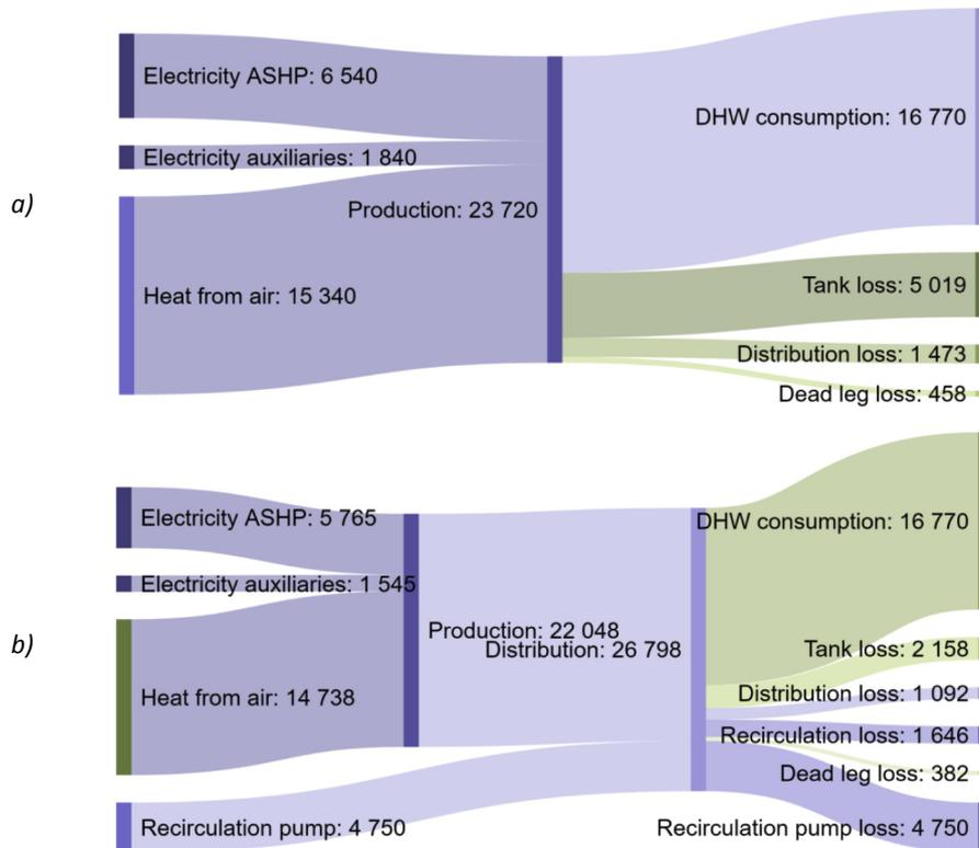
Fig. 7. Performance comparison between individual (a) and centralized (b) installation.
