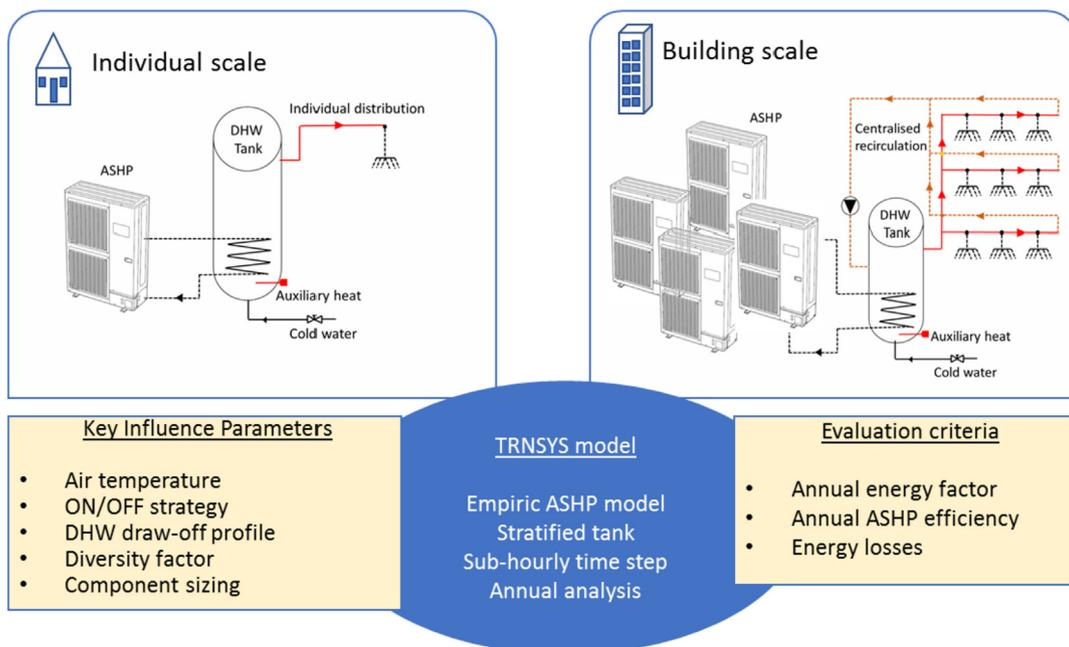
**Fig. 1.** Comparative simulation approach – what is the best heat pump integration scale for a residential need?
