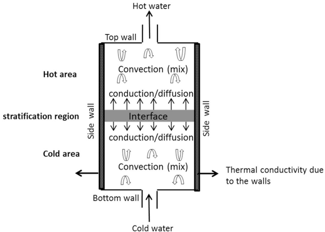
Fig. 4. Stratified hot water storage tank model.
