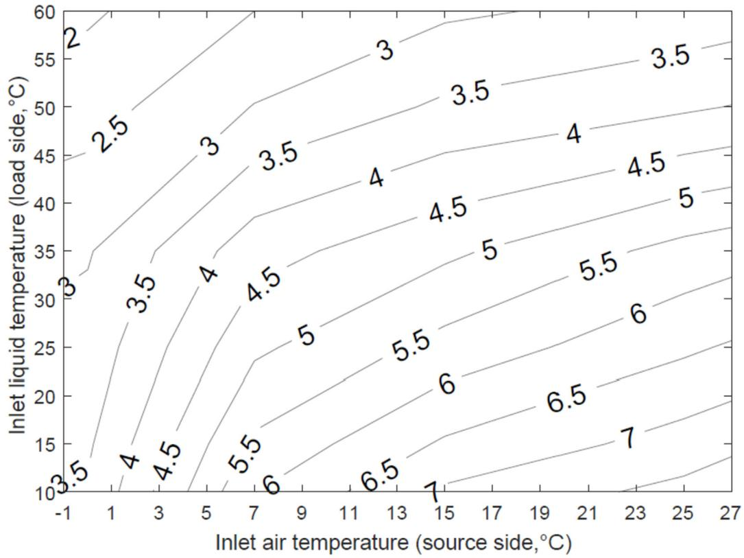
Fig. 2. COP variations as a function of hot and cold side temperatures given by the HP fabricant.
