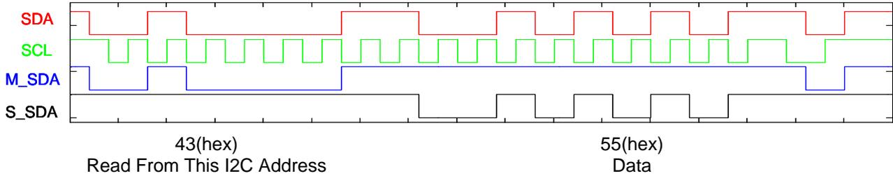
**Example 2:** This example shows how to read two bytes from the HMC6352 (slave). The slave continues to hold the SDA line low after the acknowledge bit because the first bit of the data bytes is zero.
