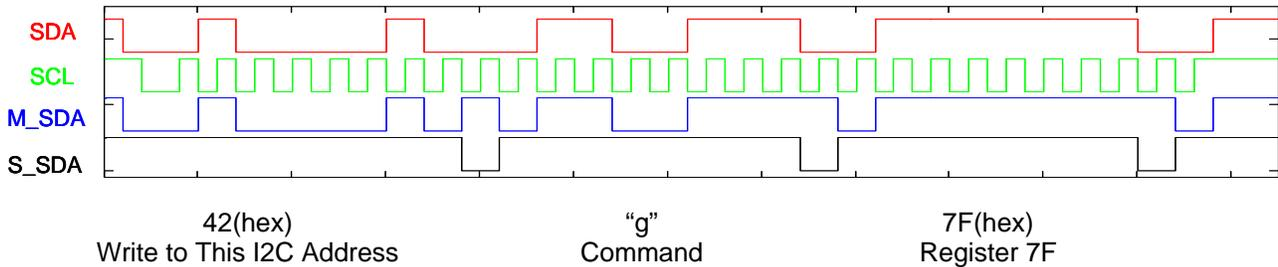
**Example 4:** This example shows how to write to a RAM register in the HMC6352 by sending the "G" command, the register address 7F(hex), and the data byte 55(hex) to the HMC6352 slave.
