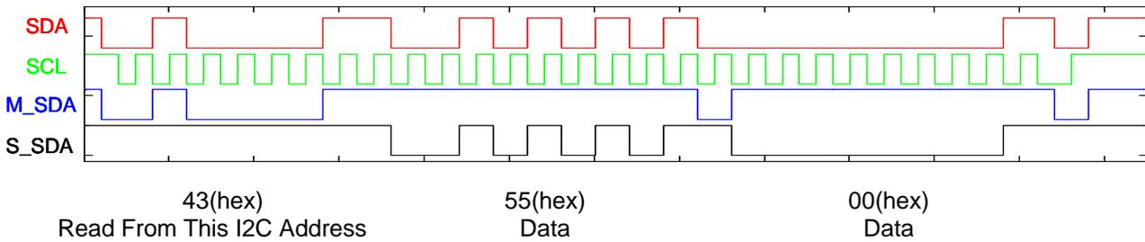
**Example 3:** This example shows how to command HMC6352 to read a RAM register by sending the "g" command and the register address 7F(hex). Note that this example does not show the process of reading the answer. See example 1 for reading a byte.
