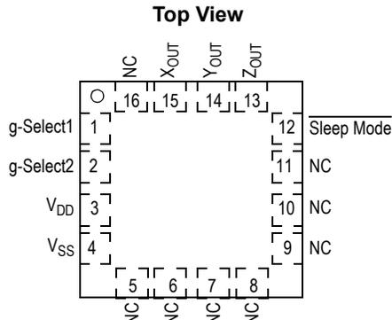
Figure 4. Pinout Description
