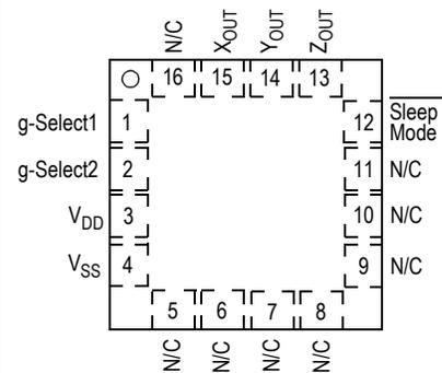
**Figure 1. Pin Connections**
