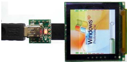
A microUSB example interface, with uUSB-MB module
