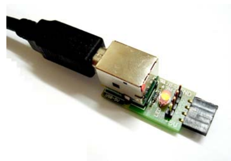
A microUSB example interface, with uUSB module
