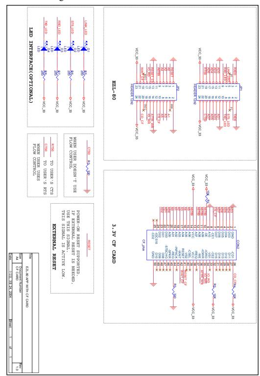
3.3.2. Interfacing circuit with a CF card
