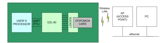
EZL-80 is a small-sized, modular product that provides TCP/IP communication through IEEE802.11b (wireless LAN) among the ezTCP product group and requires 16-bit PCMCIA card or CF card interface and a corresponding wireless LAN card.
