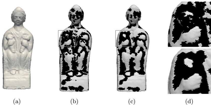
**Fig. 6.** (a) Rendering of a tridimensional mesh (*i.e.* a 2-complex embedded in  $\mathbb{R}^3$ ). (b) a threshold of the curvature map of (a). (c) Result of the operator  $ASF_{8/3}$  applied to the subcomplex shown in black in (b). (d) Crops, from top to bottom, of (b) and (c) respectively. Data courtesy of the French Museum Center for Research.
