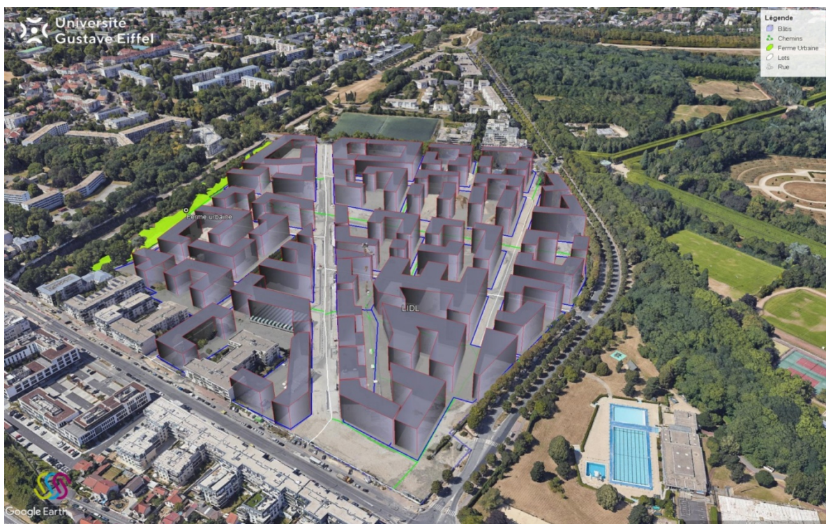
Building KML polygons drawn as 2.5models from footprint plan, displayed with Google Earth Pro
