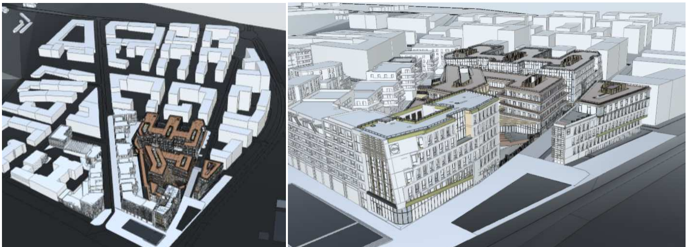
3D digital twin of LaVallée (its CIM): assembling of buildings and roads with BIM360 (Credits : Atelier M3, Arcadis, SEMOP Châtenay-Malabry - Parc Centrale )
