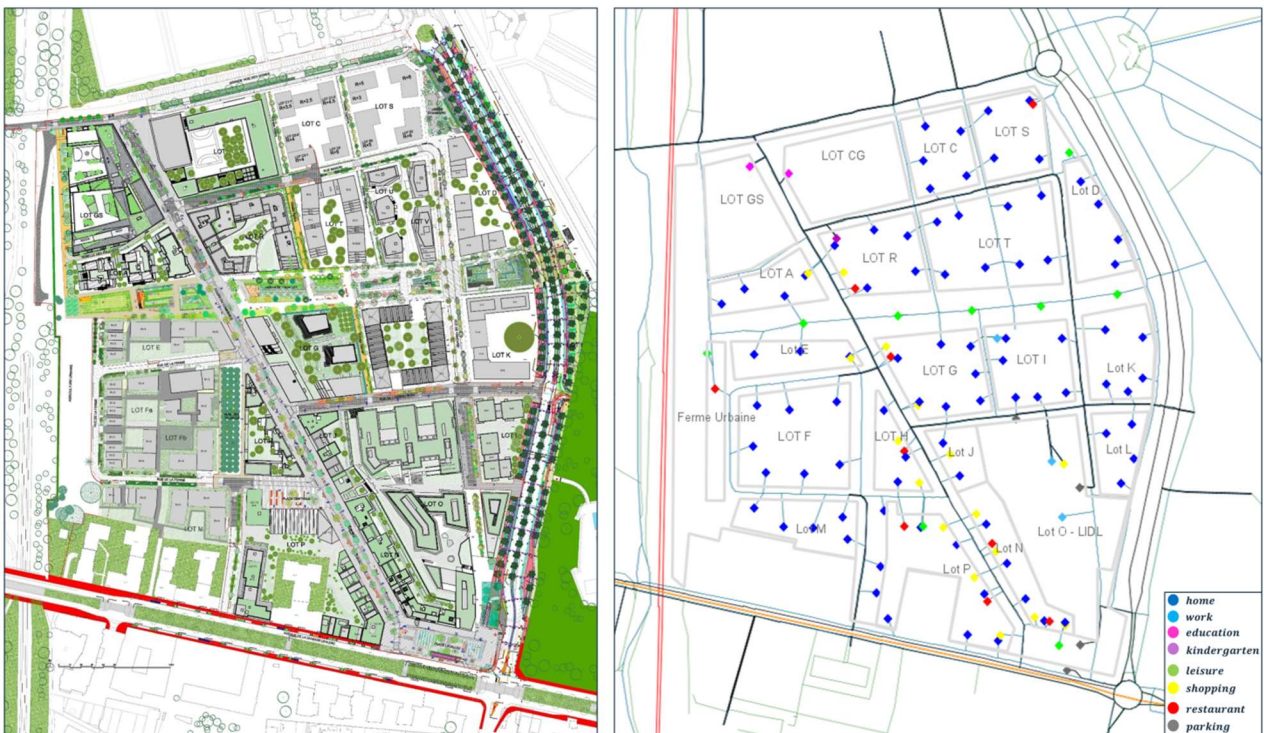
Left : Map of the road network (car/walker/bicycle) with parcels and building. Right : activities locations (Home, Work, Leisure, Shopping, Education, Restaurant and Kindergarten) with their access nodes and links to the network.
